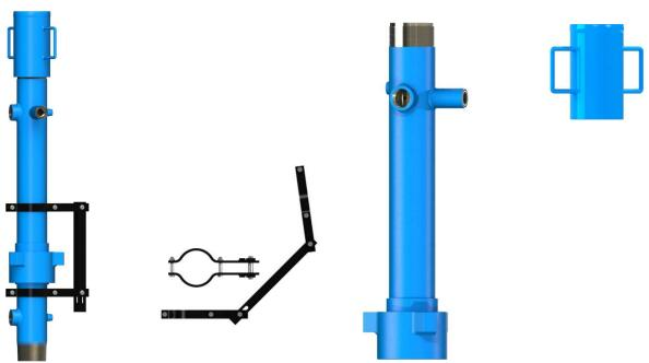
Lubricators are devices that allow the piston to stop at the end of the ascending run (they must have an adequate damping system), provide accomodation for the piston detection system (sensor) and allow to trap the piston for inspection or replacement due to exhaustion of its useful life.
