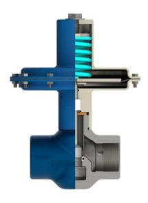
SOTEC manufactures the Model VGC-4000 valves used by the system (plunger lift) for the operation of the well. The bodies are molten in SAE 4140 steel, which have a working pressure of 4000 psi, they are subjected to hydraulic testing in an all in accordance with the standard "ASME Sect. VIII Division 1 UG-99" with a pressure of 6000 psi. It has female threaded connections in 2 "NPT (11.5 f.p.p.).
