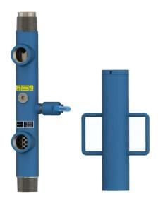
Lubricators are devices that allow the piston to stop at the end of the ascending run (they must have an adequate damping system), provide housing for the piston detection system (sensor) and allow the piston to be trapped for inspection or replacement due to exhaustion of its useful life.
